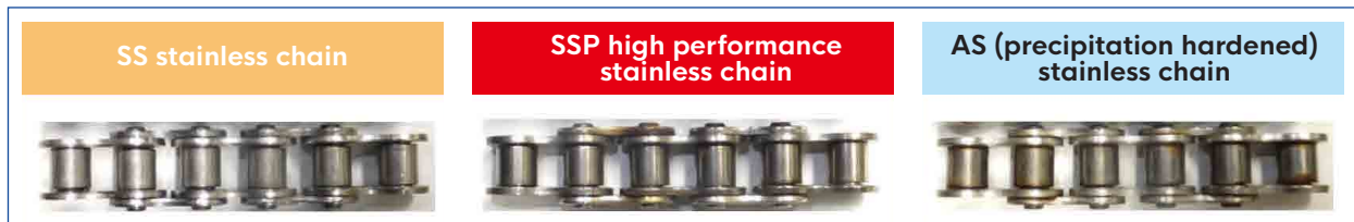
[Images of salt spray test samples after 700 hours]
